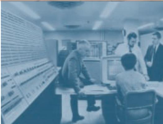
*Goddard Space Flight Center used one of two System.360 model 95 supercomputers.*
