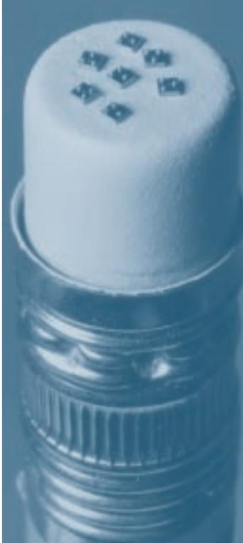
*SLT technology, scheduled for use in the System/360, would have three to six times the logical density of SMS, and 100 times more reliability. SLT chips on a pencil eraser.*
